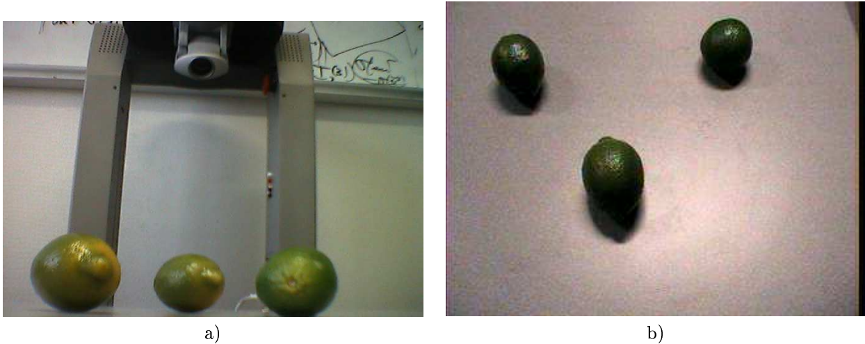
FIG. B.11 – Experimental environment : a) the PeopleBot is placed in front of a table with three green lemons. b) The image grabbed by the camera.
